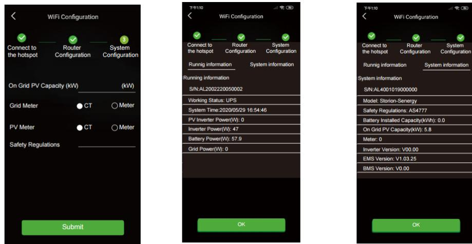
**Step 5:** Set the basic parameters, and you can see the device details. Click the "Submit" button.
